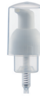
MT703 Discharge rate: 0.25 \pm 0.05 \text{ ml/T} Closure: 28/400
